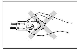
▲ To prevent reduced bulb life or cracking, do not touch the bulb with bare hands. If fingerprints are accidentally left on the bulb, wipe the bulb with a soft cloth.
