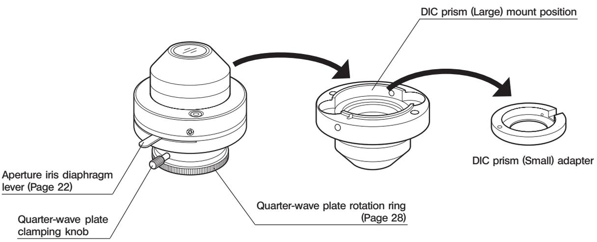
**Differential Interference Contrast Prisms (For Condenser)**
