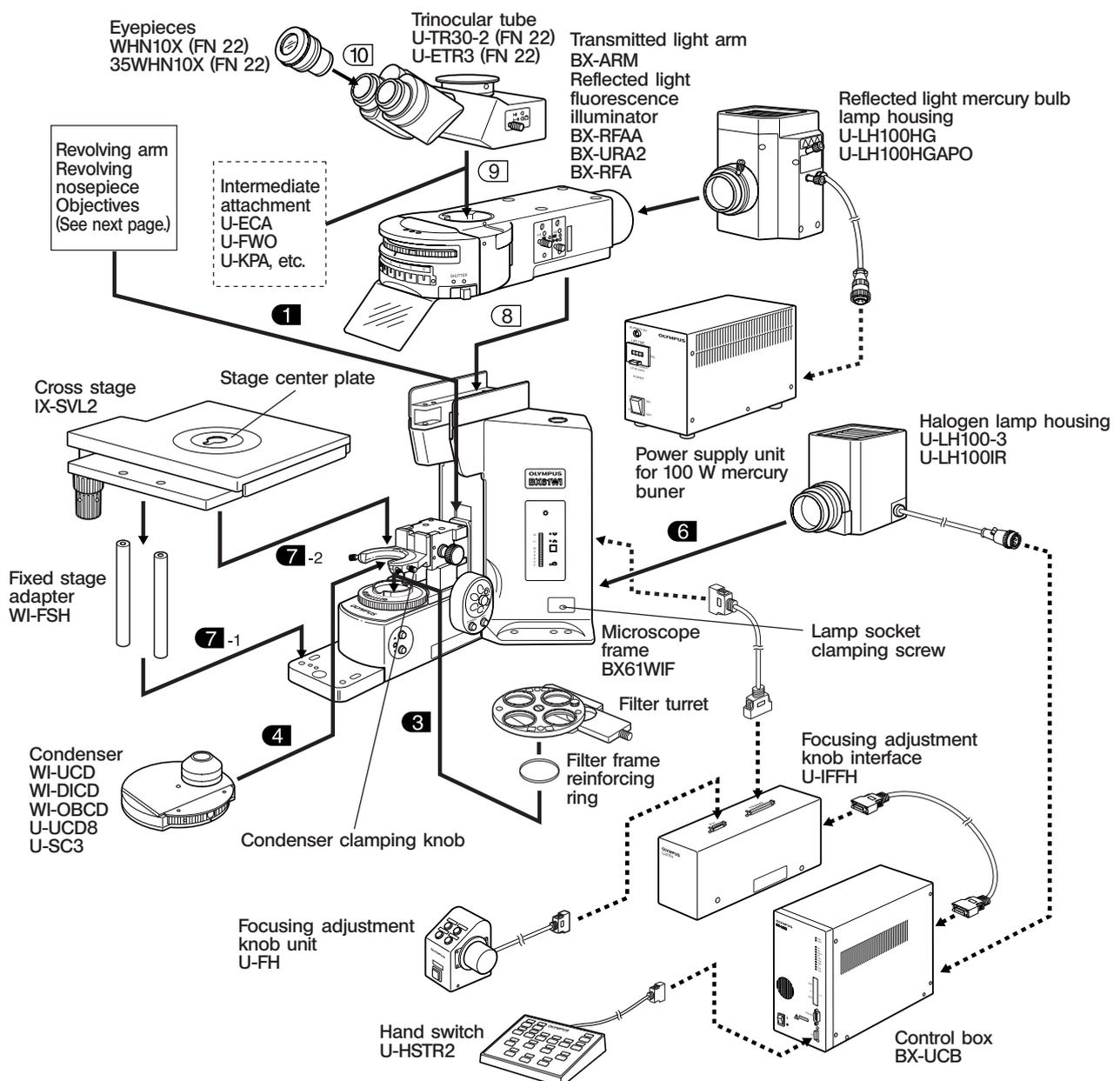
**Revolving Arm, Revolving Nosepiece, Objectives**
