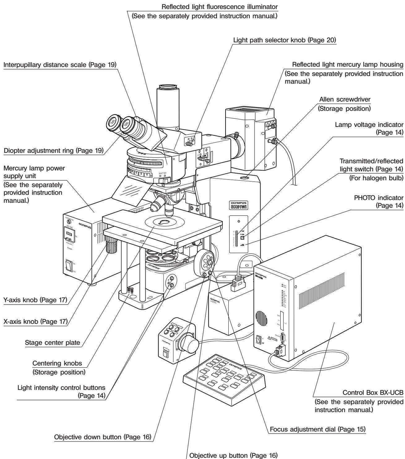
© The descriptions on the left side of the microscope frame, filter turret, revolving nosepiece, condenser, etc. will be given in the subsequent pages.
