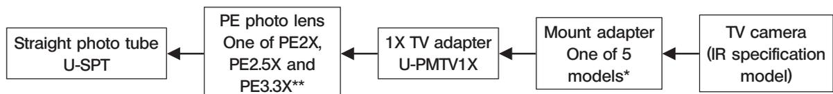
\* The mount adapter should be one of: 1) U-CMAD3 mount adapter; 2) U-BMAD bayonet mount adapter; 3) U-IMAD Ikegami camera mount adapter; 4) U-SMAD Sony camera mount adapter; 5) combination of U-FMT F/T mount + U-TMAD T-mount adapter.
