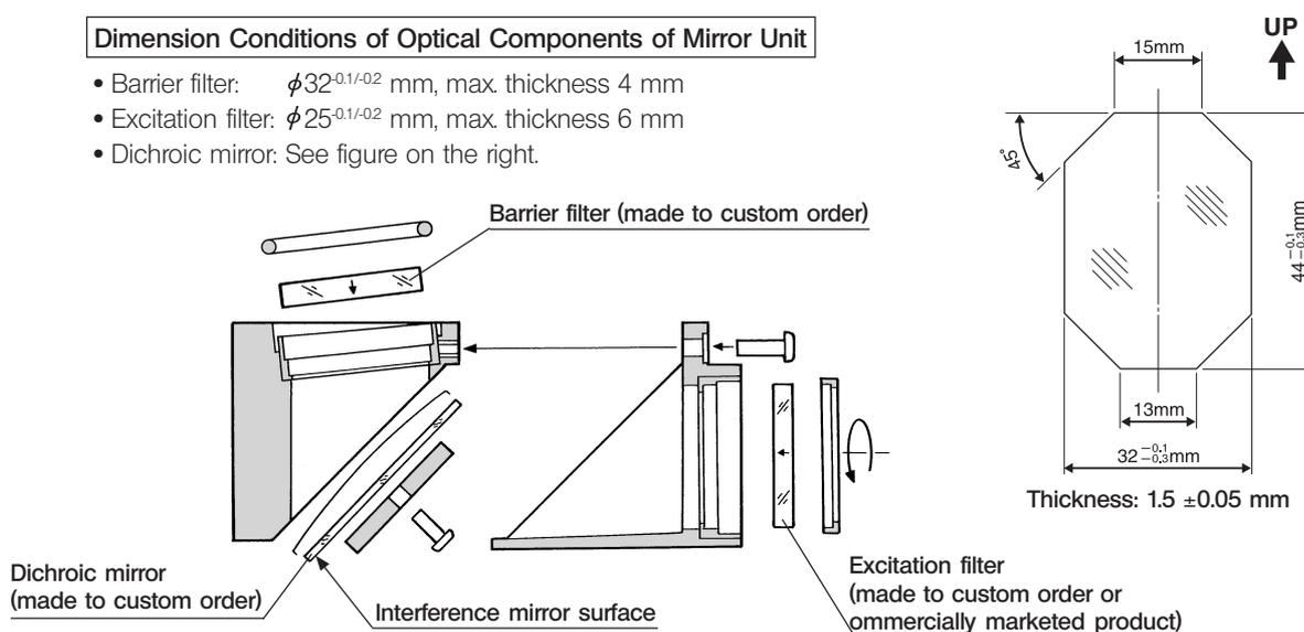
★ When replacing the dichroic mirror, take special care not to stain it by leaving fingerprints, etc.
