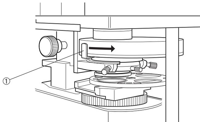
2. Then engage the IR filter (32BP775 or 32IR900) in the light path by pushing in the filter slider.
