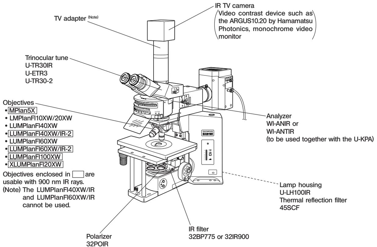
**(Note) Notes for combination of the TV adapter, intermediate attachment and observation tube**
