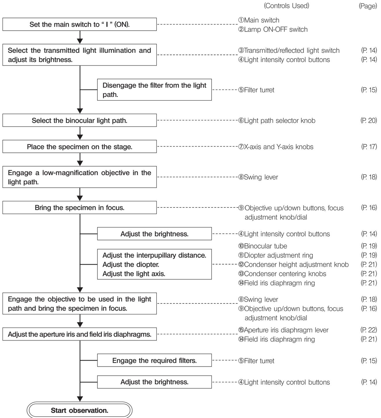
**Tip for microscope operation**
